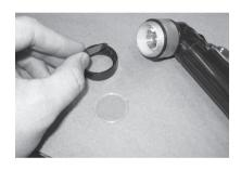
3. To change or install the lense, remove the lense cover by turning counterclockwise. Replace the existing lense with the desired lense. Replace the lense cover, and tighten by turning clockwise until finger tight.
